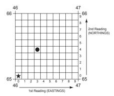
To give the six-figure grid reference, first of all identify the grid square, in this case 4665. The third figure is obtained by dividing the space between grid lines 46 and 47 into ten equal parts. Similarly the sixth figure is obtained by a similar division of the gap between northings 65 and 66. This results in a grid reference of 463654 for the dot and 460650 for the star. It should be noted that the first tenth is 0 and the last tenth is 9 in the divided grid square.
